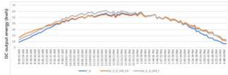
Figure 2: Example of Actual DC Energy vs. Estimated (one day, one plant, one inverter)
